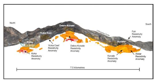
Figure 7. Long section - Koka-Konate corridor IP resistivity anomaly drill targets
