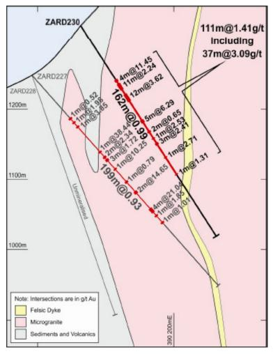
Figure 9. Cross Section Debre Konate mineralisation
