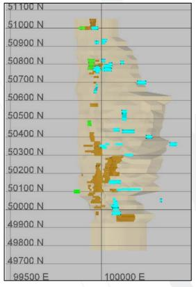
Plan View of current resource. <u>Brown areas</u> are potential block extensions not in current resource model. <u>Blue and green</u> are footwall and hanging wall mineralised zones (not included in resource model)
