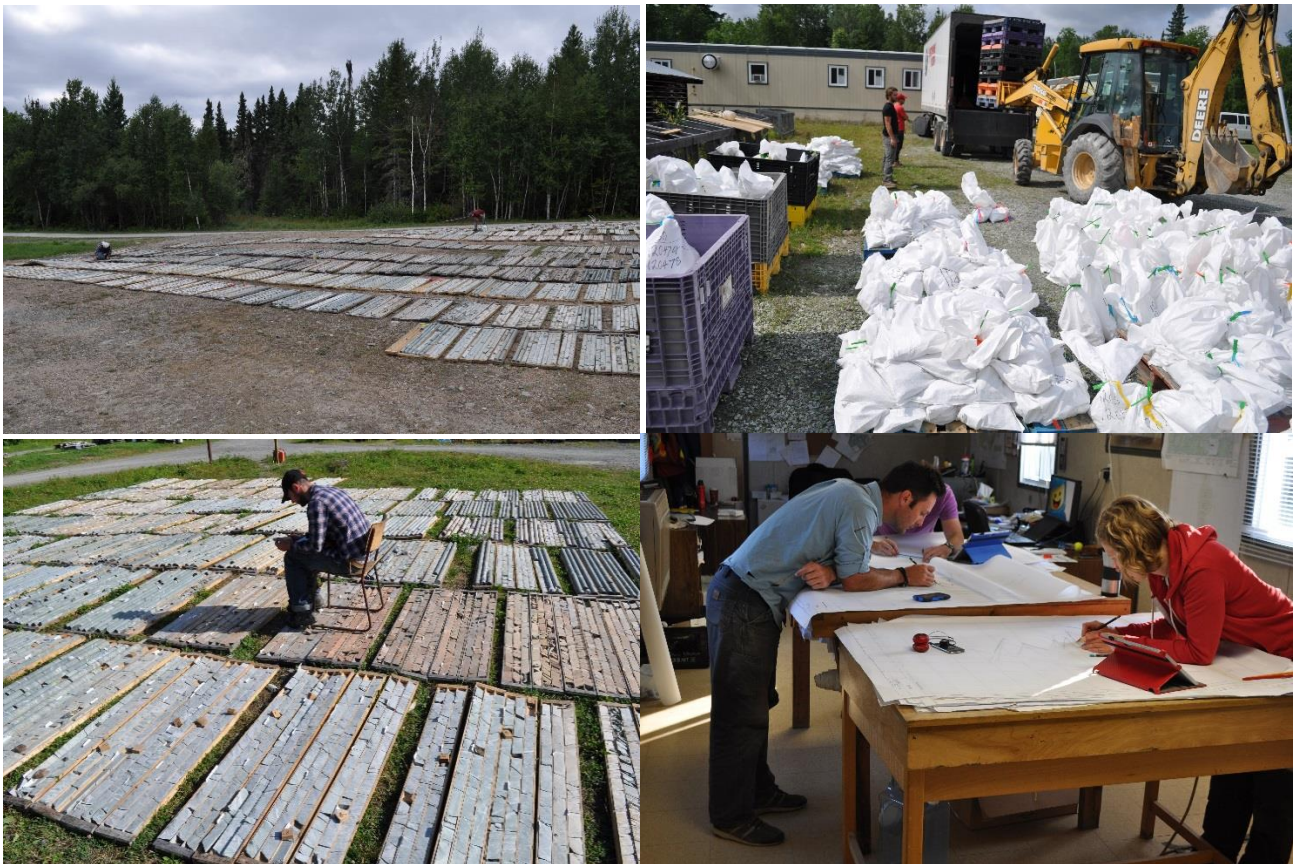
Historical core re-logging and sampling (top left – core laid out for logging; top right – samples being dispatched to assay lab; bottom left – geological logging; bottom right – cross section interpretations)
