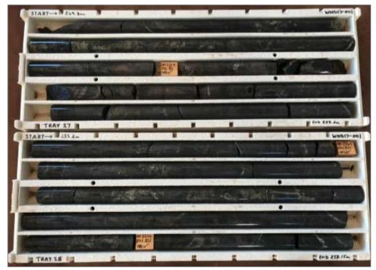
**Figure 3.** Diamond Hole WND17-001 – 249.3-258.15m showing strong magnetite-ironstone with chalcopyrite mineralisation.
