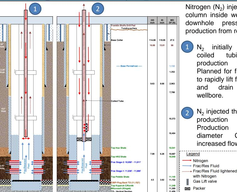
Nitrogen  $(N_2)$  injected to lighten fluid column inside wellbore and reduce downhole pressure to improve production from reservoir.
