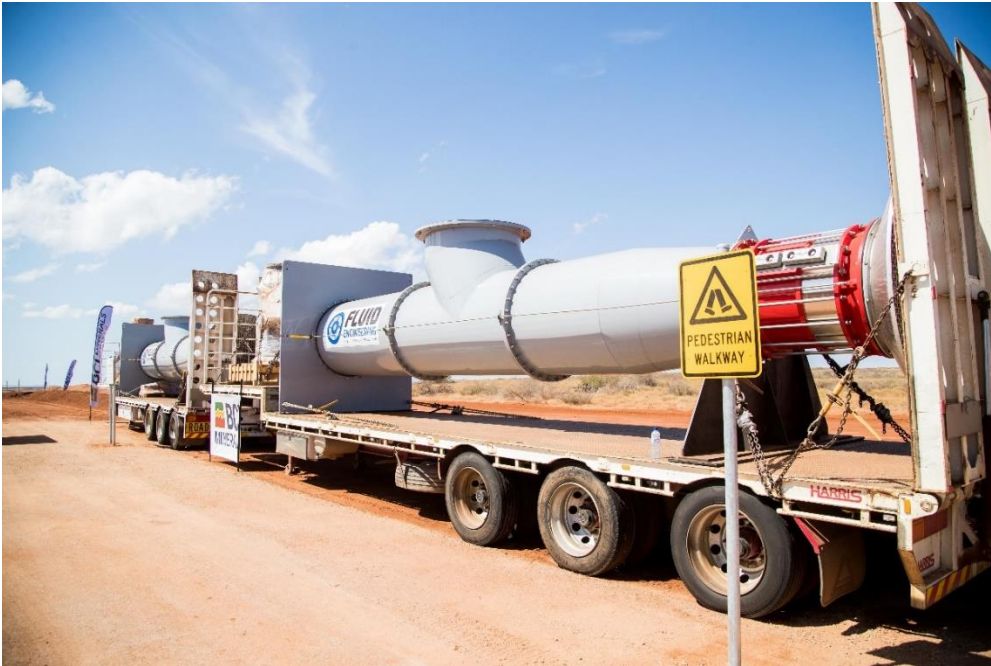
Two of six primary seawater intake pumps arriving at Mardie Site
