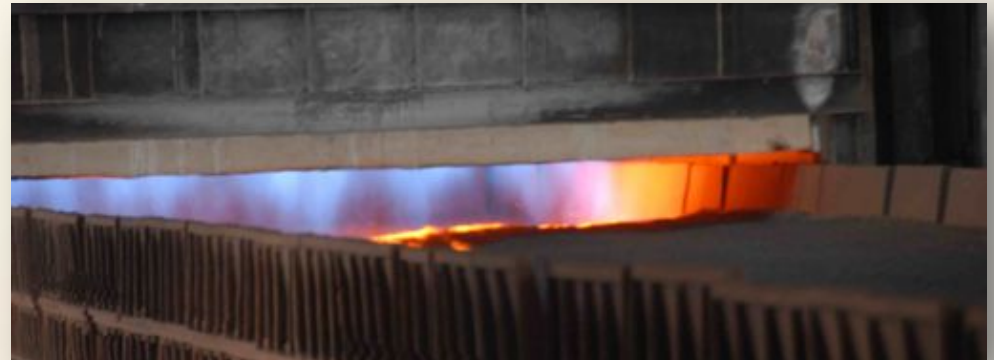
Ignition hood on sinter strand
