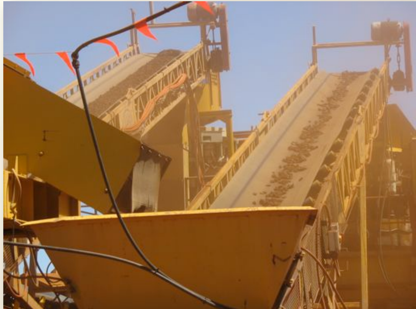
Simple secondary screening and crushing circuit
