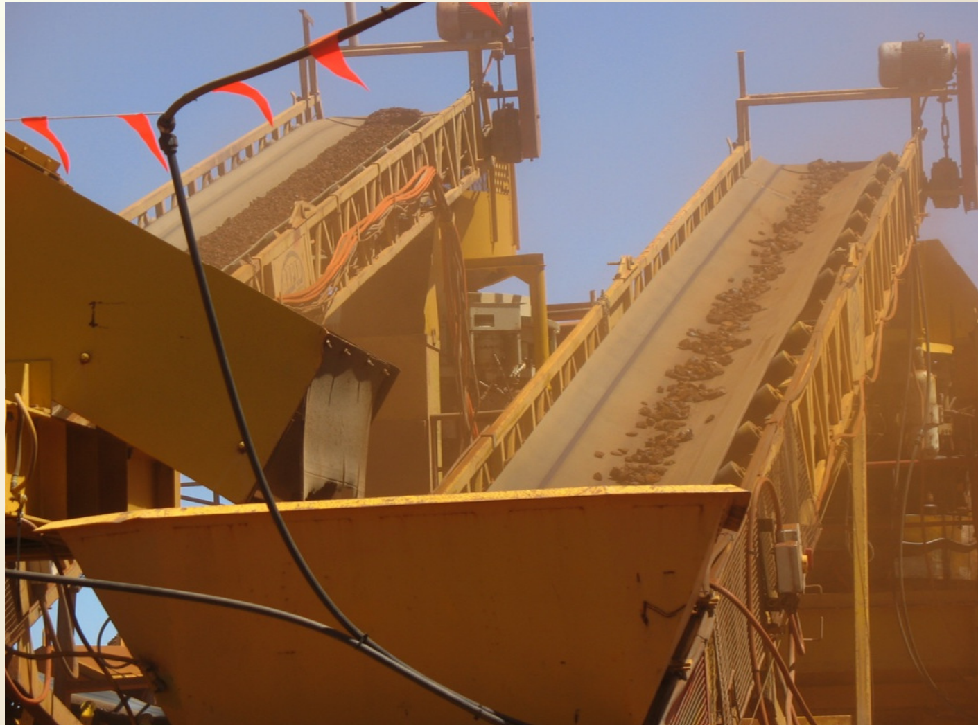
Simple secondary screening and crushing circuit
