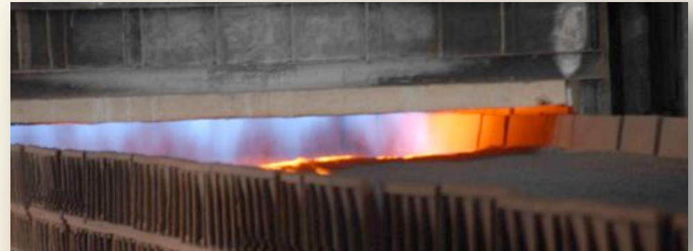
Ignition hood on sinter strand
