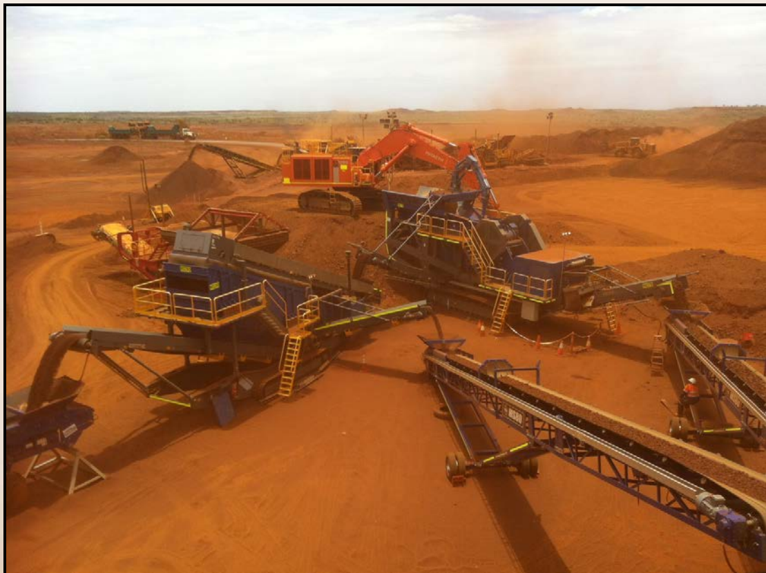
Figure 2: Kleeman scalping circuit at site
