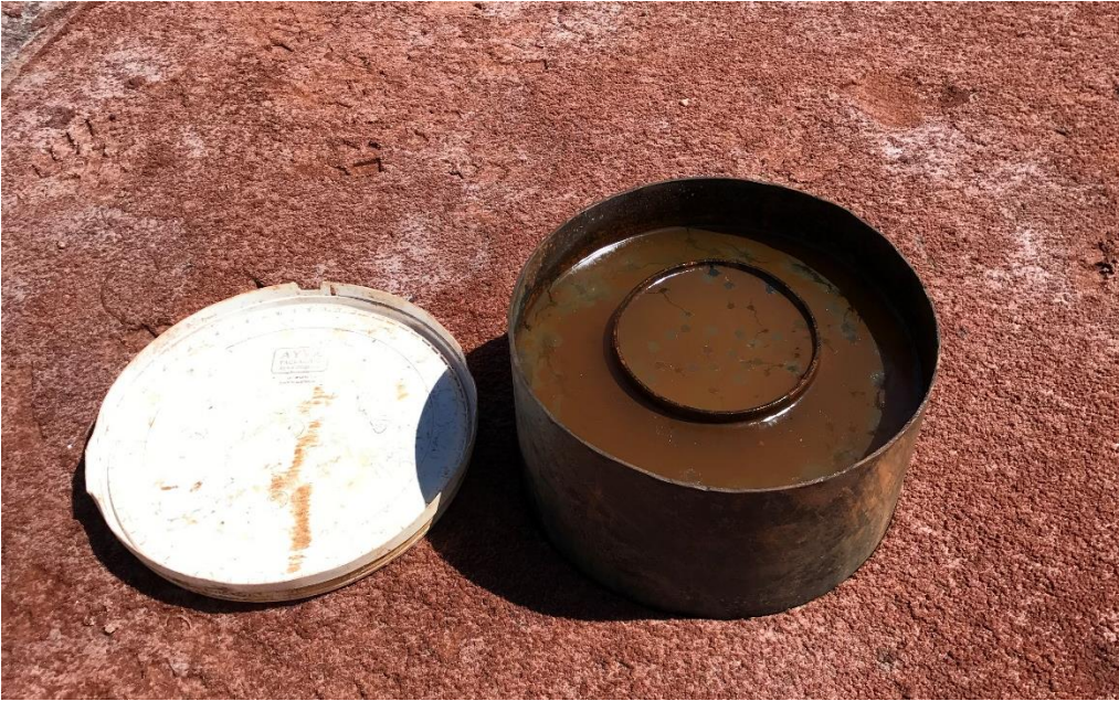
Figure 3: Geotechnical Investigations (Double Ring Infiltration Tests)
