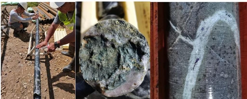
Image 1. (Left) – Cleaning the core at the split tube prior to transfer to core boxes. (Centre) – Core photo at ~190 metres depth, assays awaited. (Right) – Core photo at ~200 metres depth, assays awaited. Core is HQ sized and has a diameter of 63.5mm
