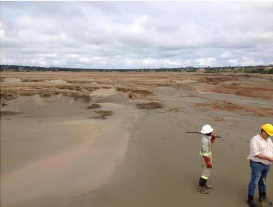
**Issue** | The tailings at several mines in the region contain copper and zinc at grades that are uneconomic to process using conventional approaches. One identified mine alone contains \$1billion+ of potential recoverable value. These tailings present a significant environmental problem with potential to leach metals and an economic opportunity for metal extraction.
