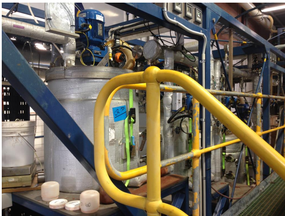
Figure 6: Clean TeQ Pilot Plant: Leached Pulp Neutralisation Circuit
