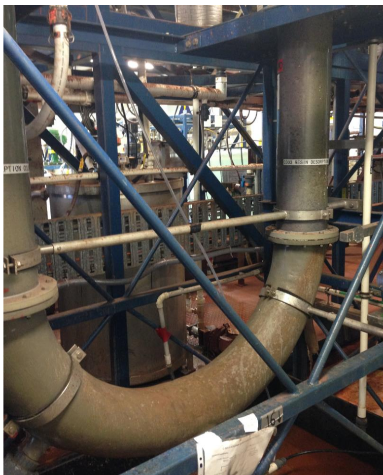
Figure 7: Clean TeQ Pilot Plant: 'U-Column' Nickel/Cobalt Recovery System
