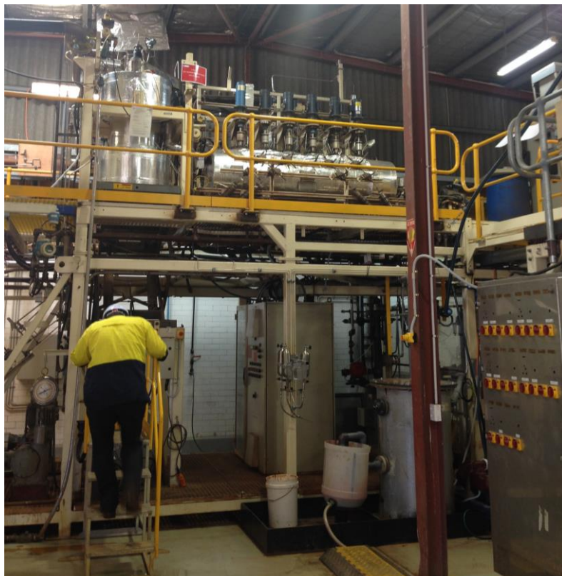
Figure 5: Pilot Plant: High Pressure Acid Leach Autoclave (horizontal cylinder at top of photo)
