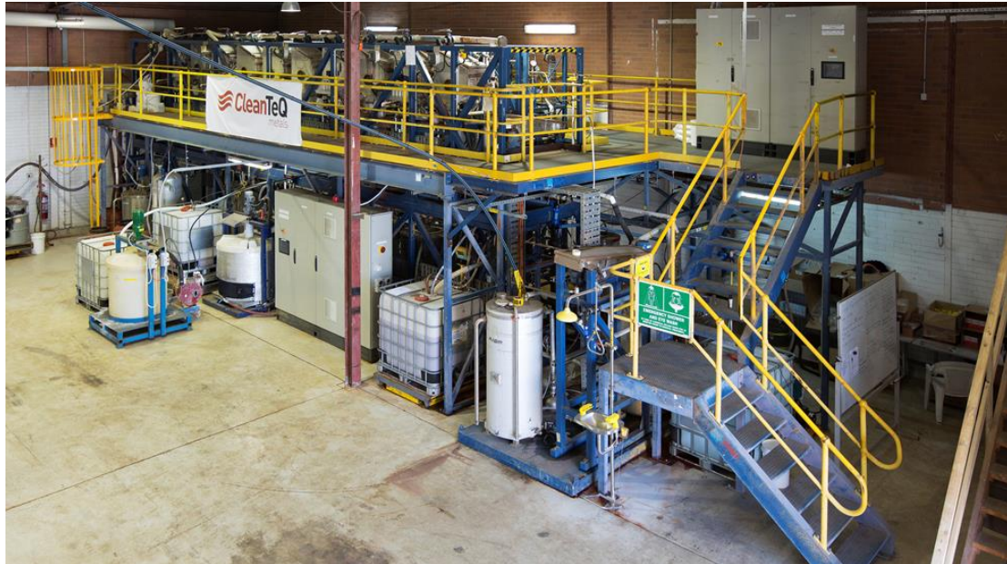
Figure 4: Clean TeQ's Proprietary Resin-In-Pulp (cRIP) Pilot Plant
