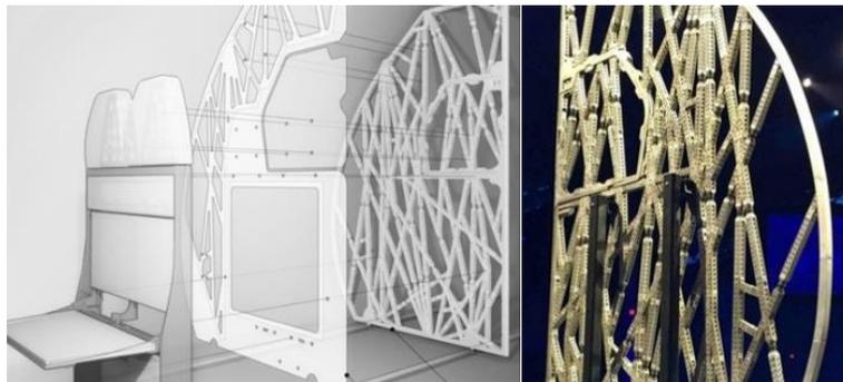
**Figure 3: 3D Printed Scalmalloy<sup>®</sup> RP partition and Aleris creep formed AlMgSc part**
