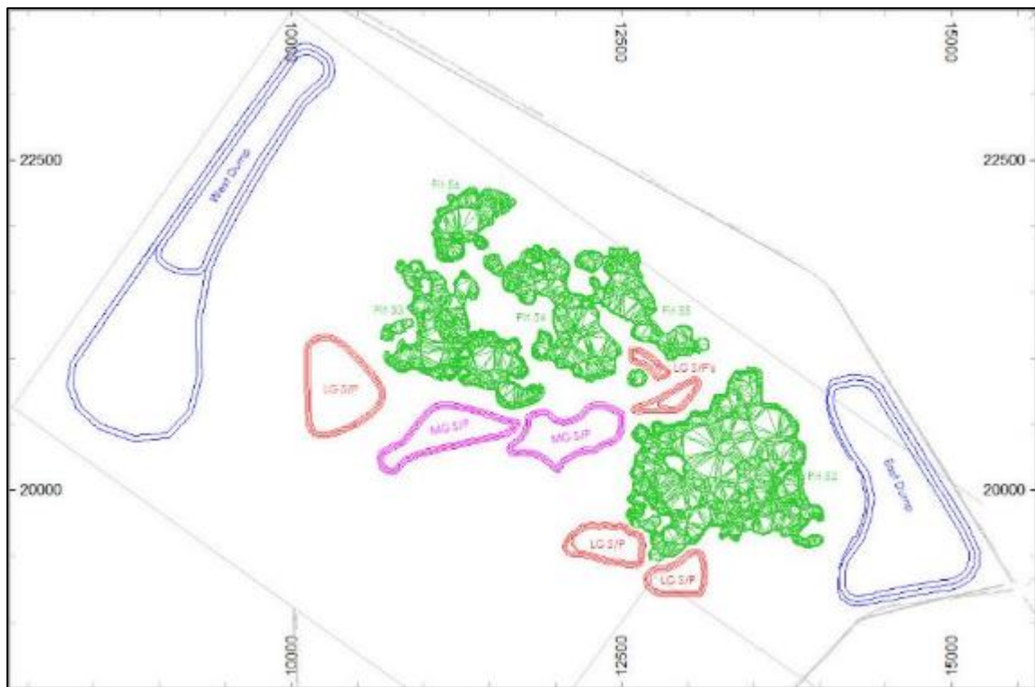
Figure 16-3: Pit, stockpile and waste dump design – Year 10
