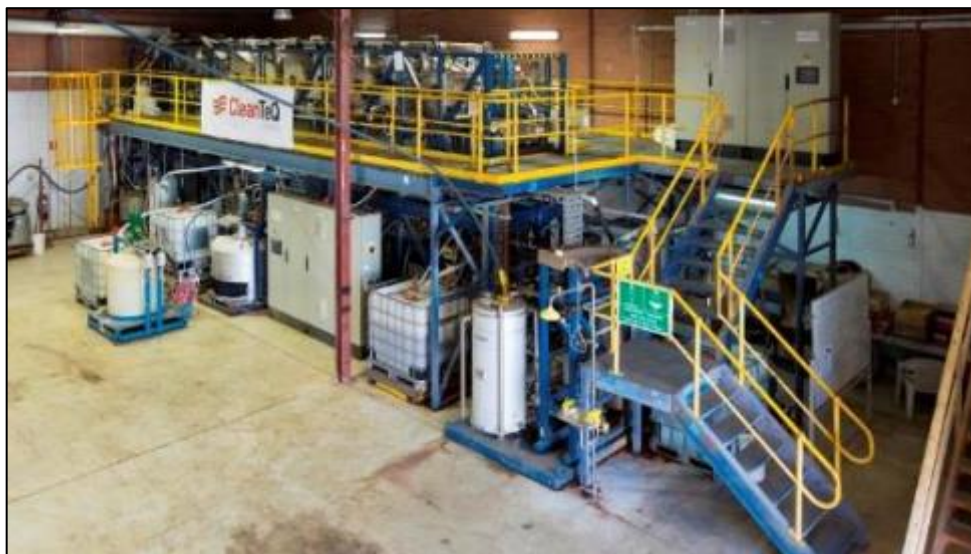
Figure 13-4: Overview of laterite scandium extraction RIP pilot plant
