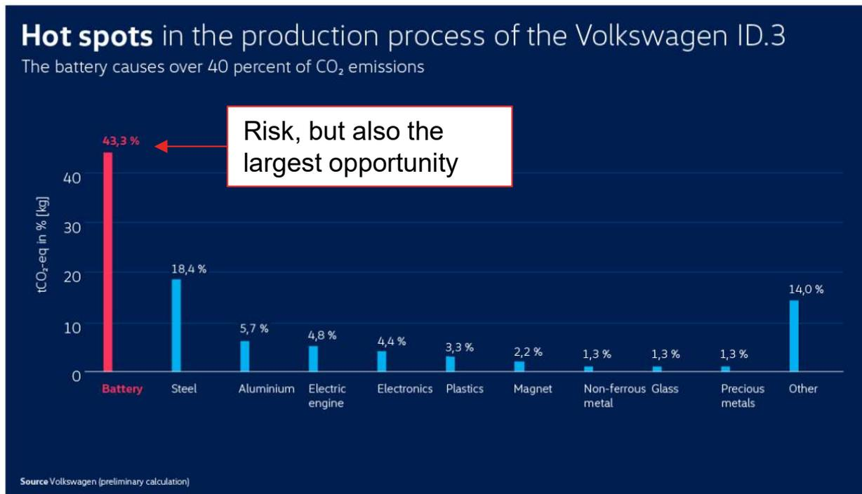
Raw materials (mining and processing) in the battery leave the biggest CO<sub>2</sub> footprint on the supply chain
