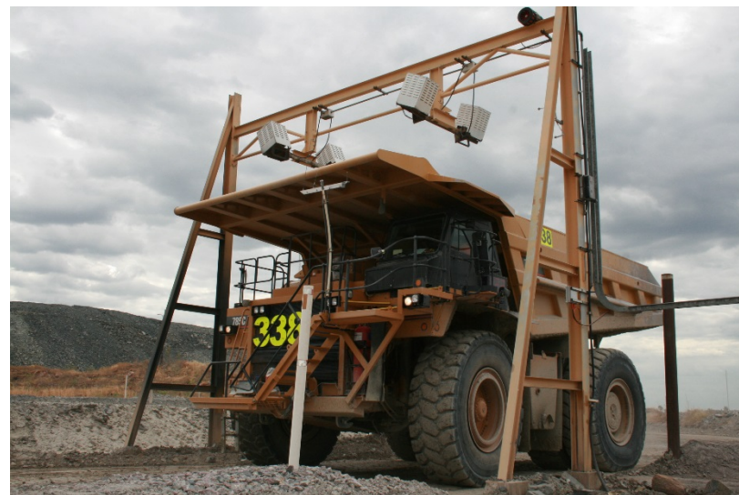
Mine truck under the discriminator
