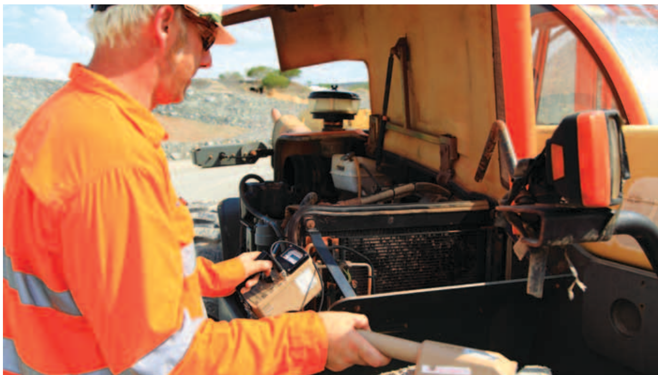
Andrew Calcott, Radiation Safety Advisor, undertaking a radiation check prior to the vehicle leaving Ranger mine.
