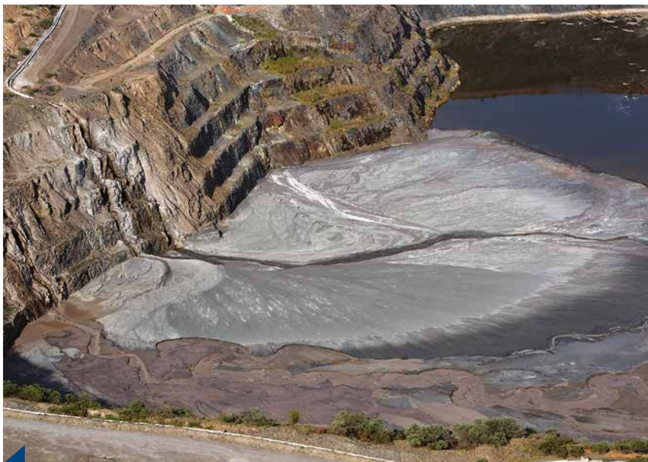
A beach is forming in Pit 3 as tailings are deposited via pipelines from the Tailings Storage Facility and the mill.
