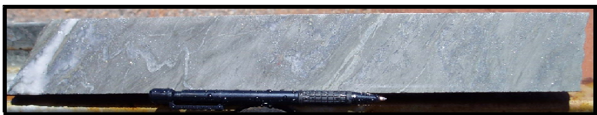
Figure 2: SPDD2 Core Sample 207.8m - 208.2m. Interval grade 9.6g/t
