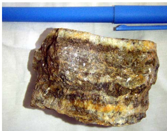
Silver-rich banded vein with crustiform quartz & minor pyrite
