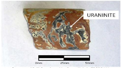
Segment of Drill Core from 98m Down Hole in TPCDD006
