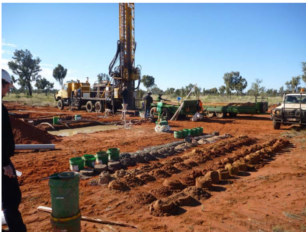
Mud-Rotary Drilling at Ngalia Basin in 2010
