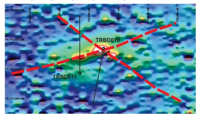
Figure 4. Impaler ground magnetics anomalies with historical drill collars and interpreted structures.
