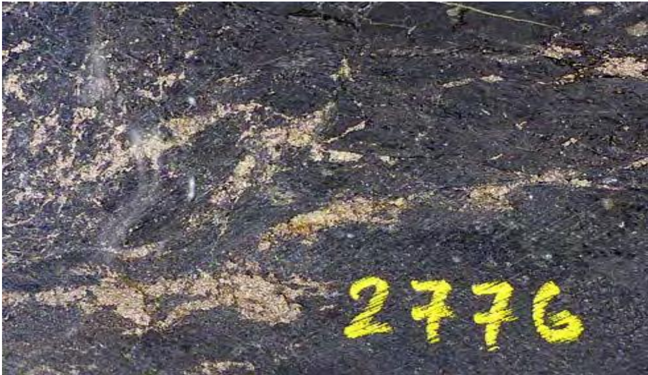
Core from 168.8m in TALDD001 showing graphite with sulphides (pyrrhotite, pyrite) in quartz-muscovite schist. Field of view approximately 3 cm.
