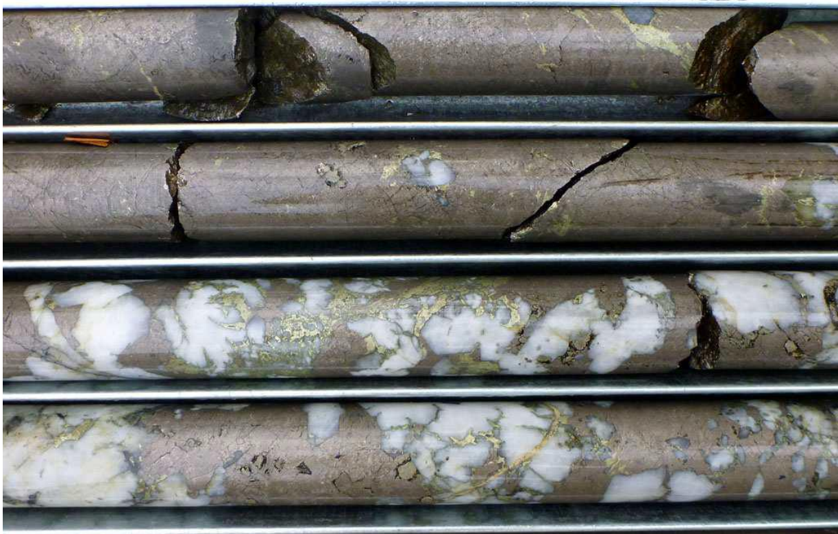
Massive sulphides (pyrrhotite; blebby chalcopyrite) and quartz-chalcopyrite breccia. TALRCDD003 (156-161m)
