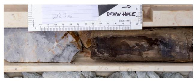
Figure 5. Crown Prince: wooden core from unmapped old stopes at 112.7m in TGGDD086.
