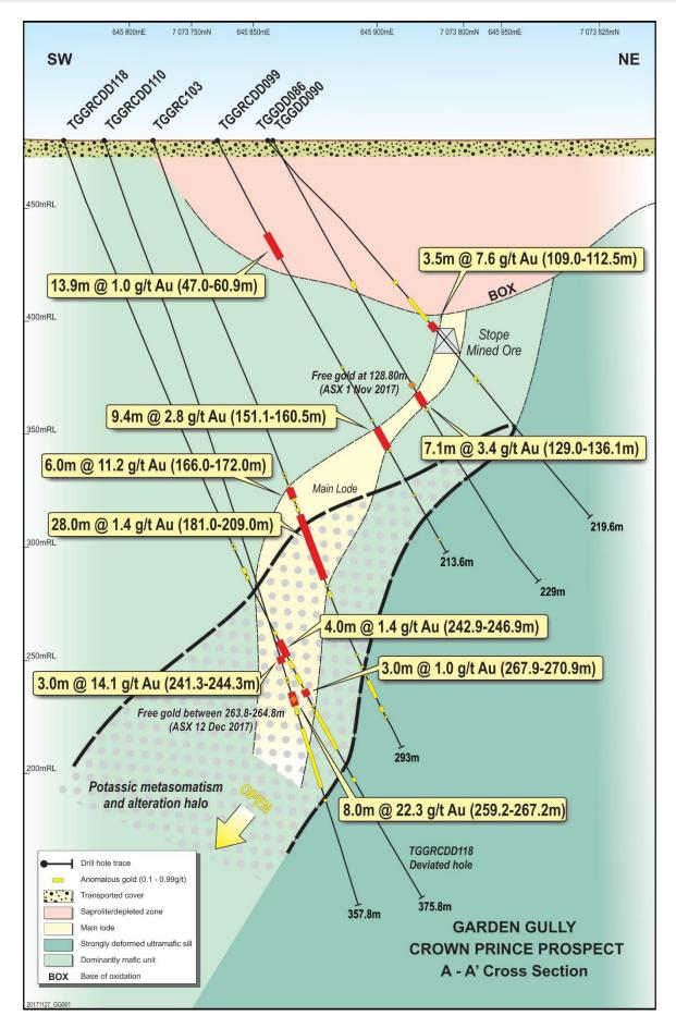
Figure 4. Crown Prince Prospect. Cross section A-A' through the Main Lode, looking north-westerly.
