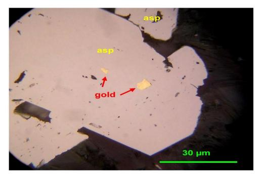
Figure 7. Gold inclusions in arsenopyrite (asp). TGGDD090, 135.02m downhole.
