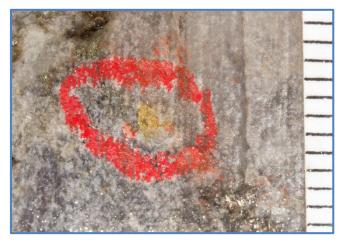
Figure 13. Free gold and sulphide at 264.80m.
