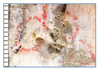
Figure 11. Free gold and sulphide at 264.10m.
