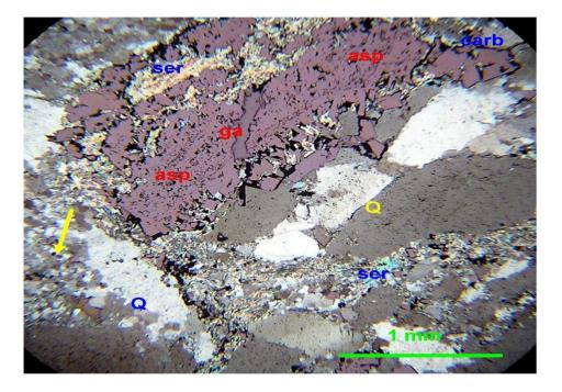
Figure 6. Late-stage galena (ga) carrying high silver values, cross-cutting arsenopyrite (asp). Sample taken from 131.05m downhole in TGGDD090.
