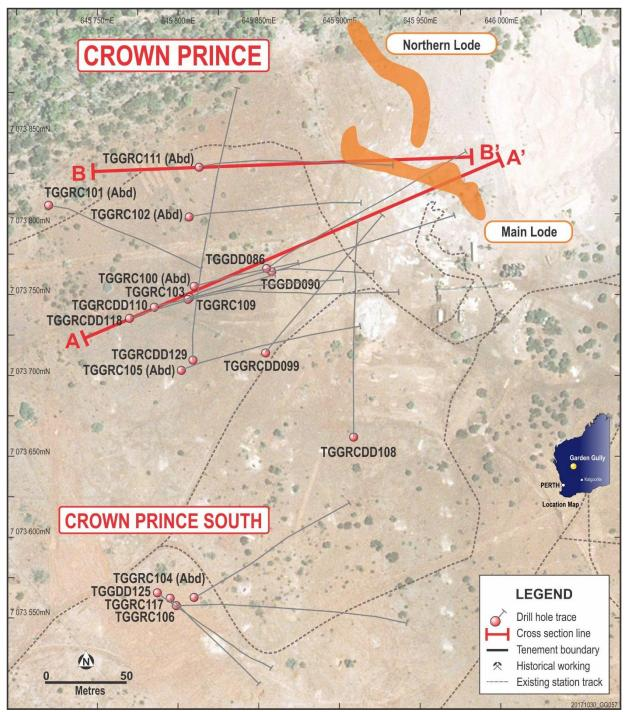
Figure 3. Distribution and surface projection of drill hole traces at Crown Prince Prospect.
