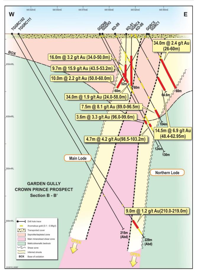
Figure 15. Inferred down dip / plunge extensions of Main and Northern Lodes (B-B' section on Figure 4).
