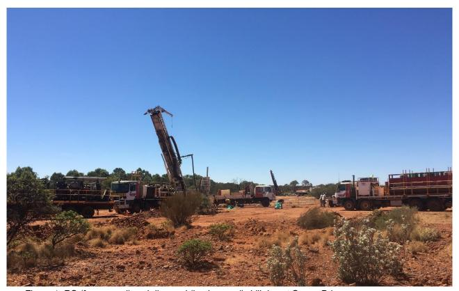
Figure 1. RC (foreground) and diamond (background) drill rigs at Crown Prince.
