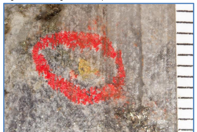
Figure 15. Free gold and sulphide at 264.80m.
