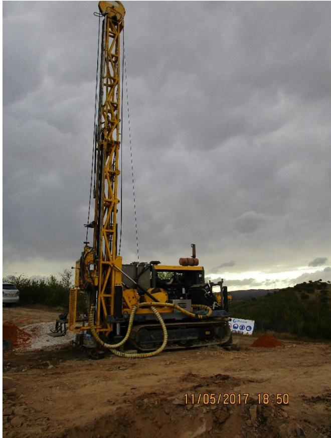
The Drillcon Iberia diamond drill rig completing set-up on site for the first hole of a 5 hole program at Auroch's Alcoutim Project.
