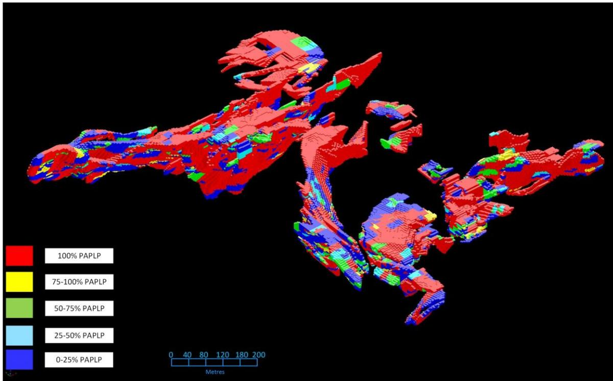
**Figure 2: Pit Shells showing Scheduling Stages (at Year 10)**
