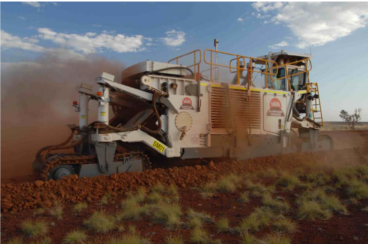
Vermeer 1255T (above) and Wirtgen (below) surface miners commence cutting at the Outcamp deposit yesterday
