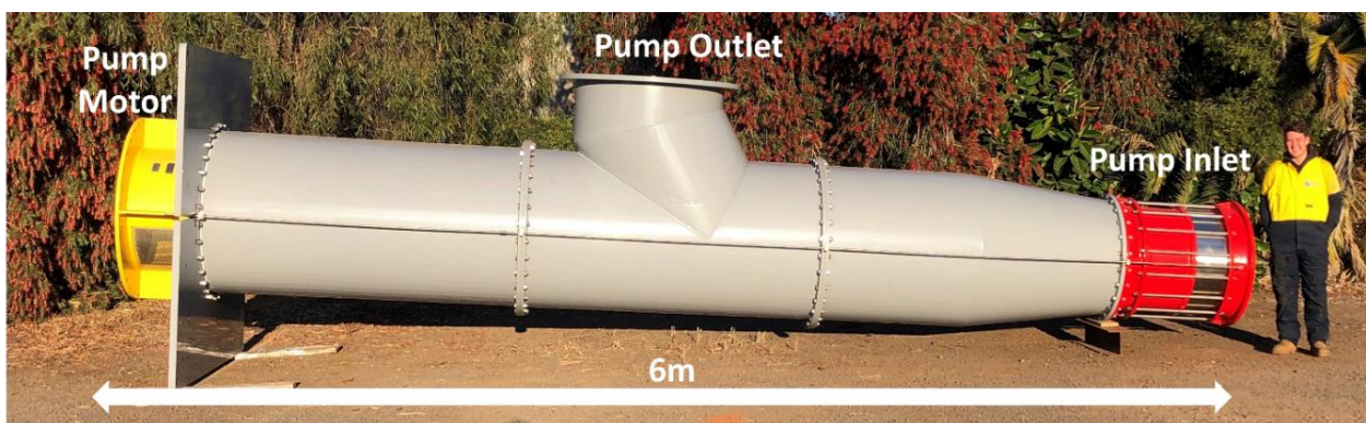
Figure 1: Seawater Intake Pump
