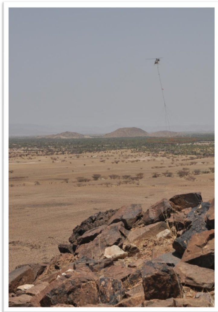
Figure 4: Aerospatiale Lama helicopter with suspended Geotech VTEM and magnetic systems
