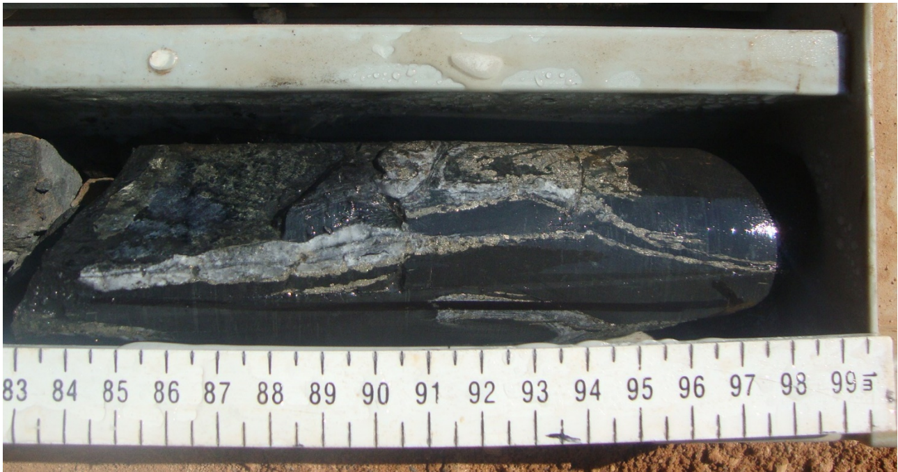
Figure 3: Close up of sulphides in core.
