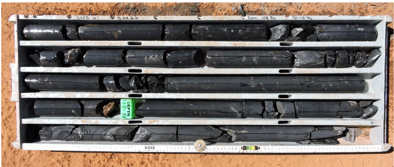
Figure 2: Diamond Core Sample for Metallurgical Testwork.
