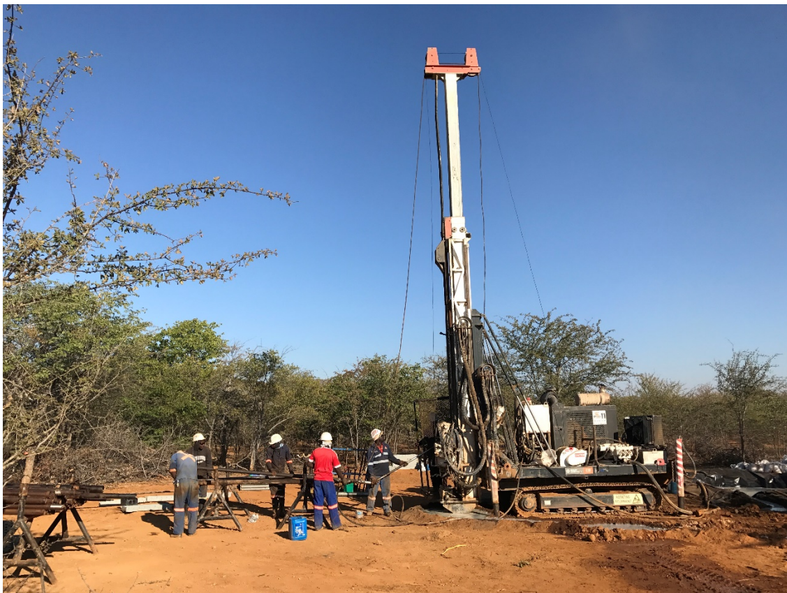
Figure 4: Diamond Drilling in progress.
