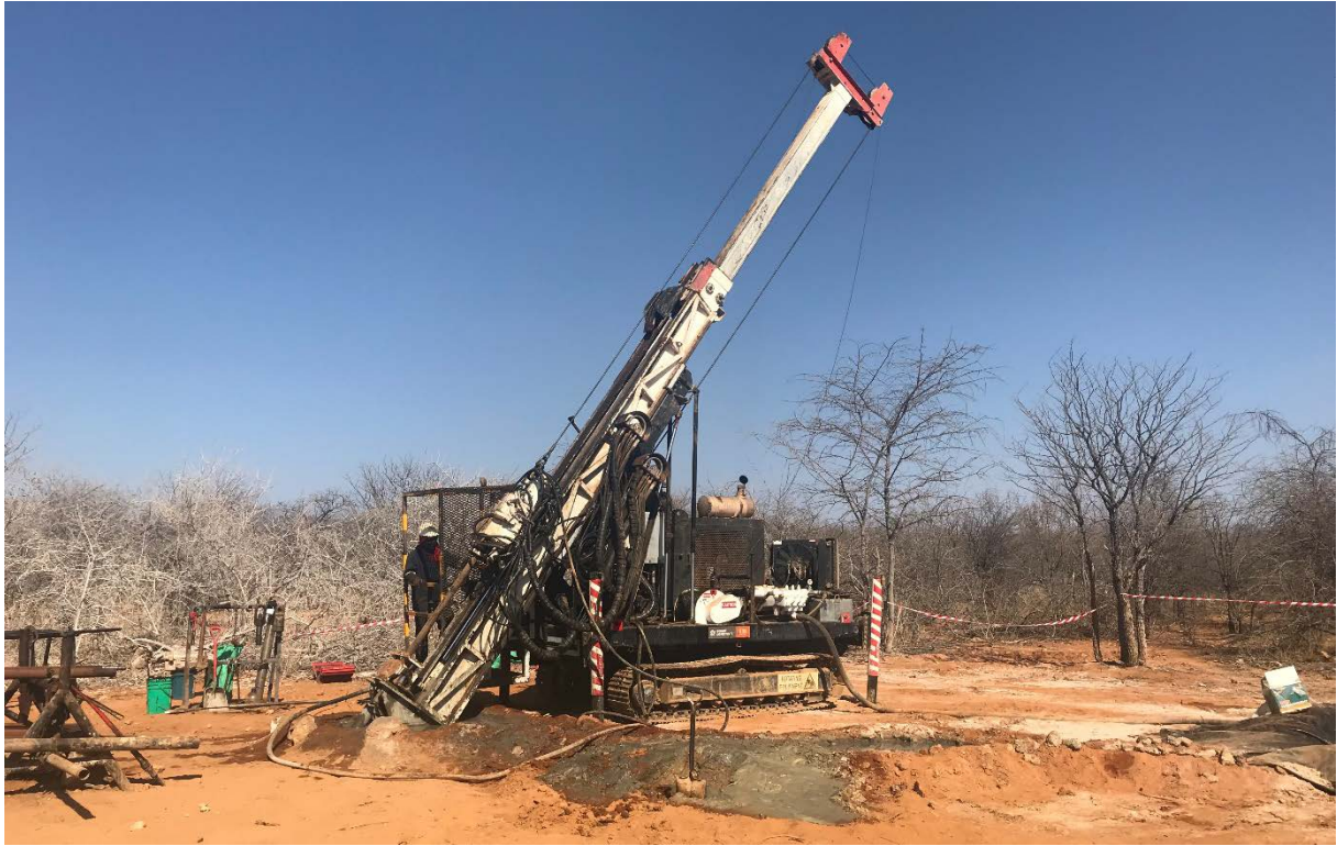
Figure 2: Diamond drill rig operating at the Project
