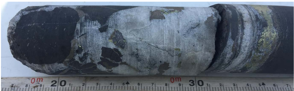
Figure 5: DOFD0077 (492.95 m) - Chalcopyrite-sphalerite-pyrrhotite-linnaeite sulphide mineralisation
