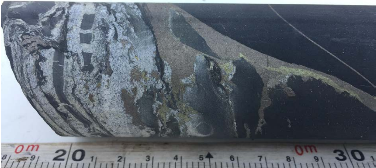
Figure 4: DOFD0077 (492.4 m) - Chalcopyrite-sphalerite-pyrrhotite-linnaeite sulphide mineralisation
