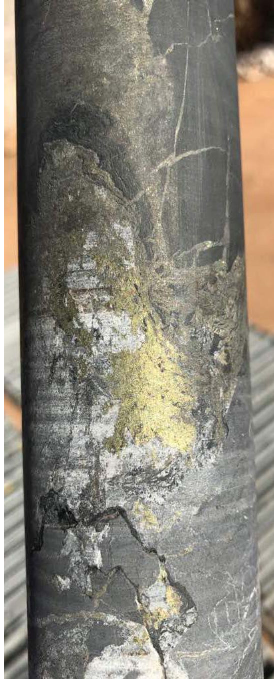
Figure 7: Sulphide Mineralisation in Drillhole DOFD0114 (Approximately 435 m Downhole)
