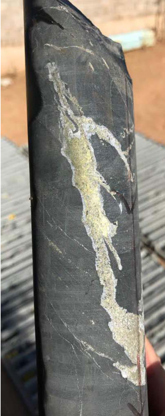
Figure 6: Sulphide Mineralisation in Drillhole DOFD0114 (Approximately 435 m Downhole)
