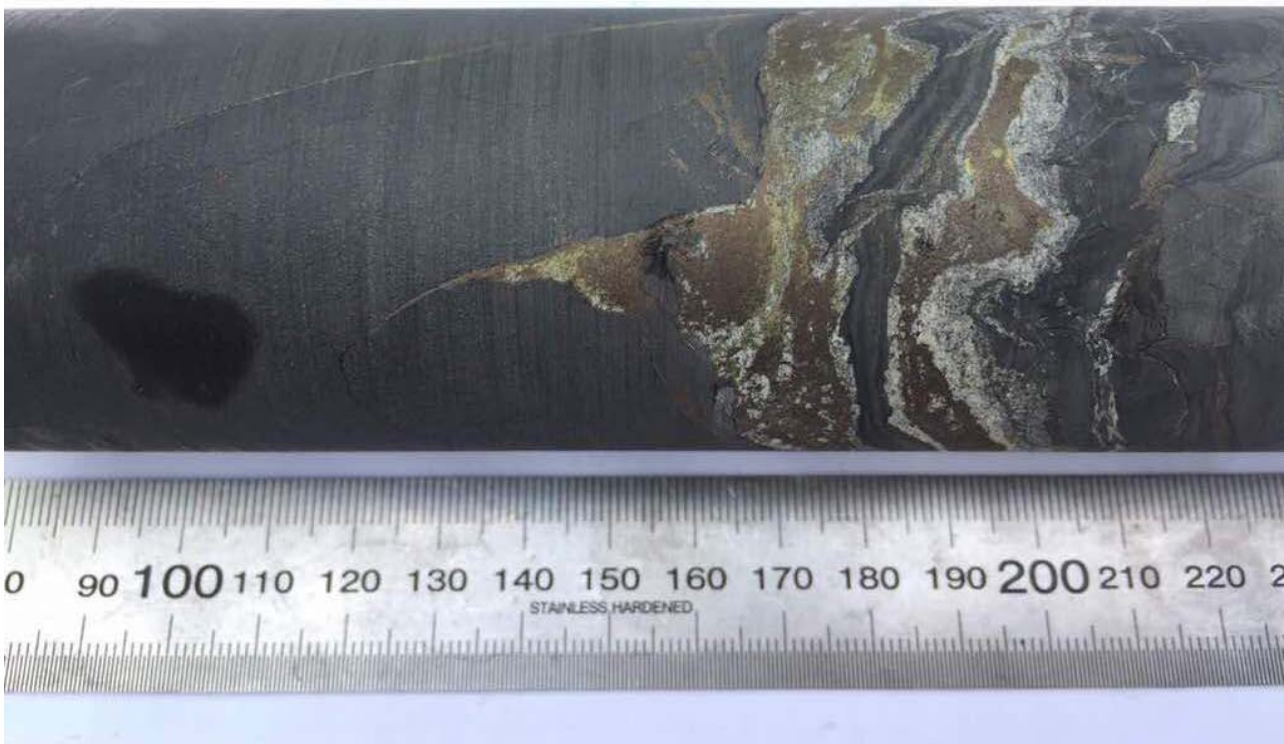
Figure 5: Sulphide Mineralisation in Drillhole DOFD0103 (Approximately 450 m Downhole)
