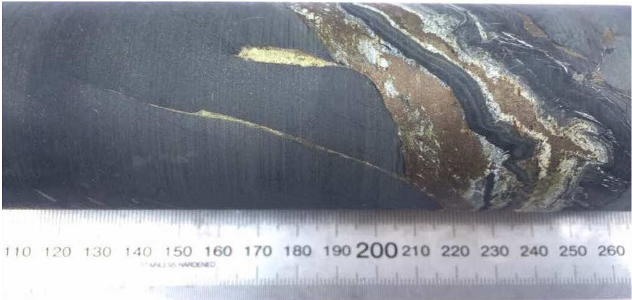
Figure 4: Sulphide Mineralisation in Drillhole DOFD0103 (Approximately 450 m Downhole)
