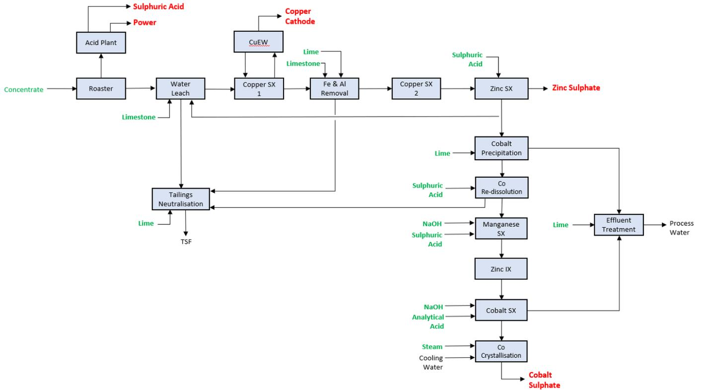
**Figure 4: Preliminary Autoclave Leach Option Flowsheet**
