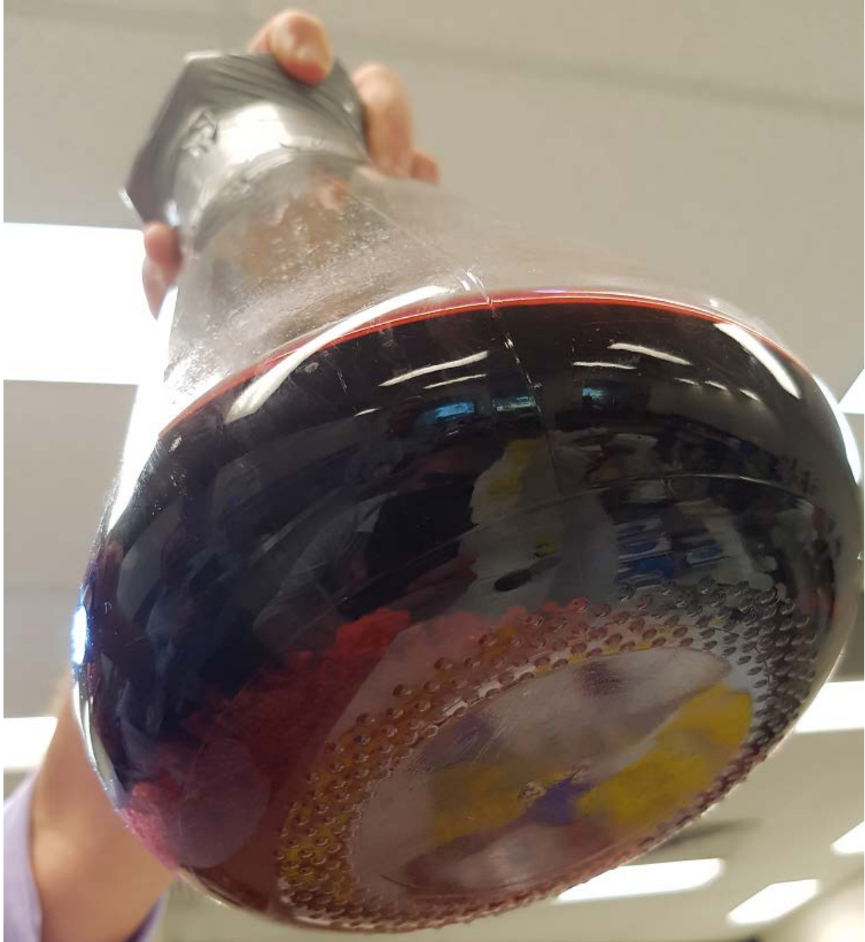
Figure 4: Cobalt sulphate solution with cobalt sulphate crystals visible at the base of container
