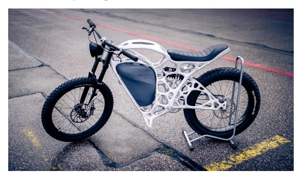
The world's first 3D printed electric bike aluminiumscandium frame makes it lighter and stronger
