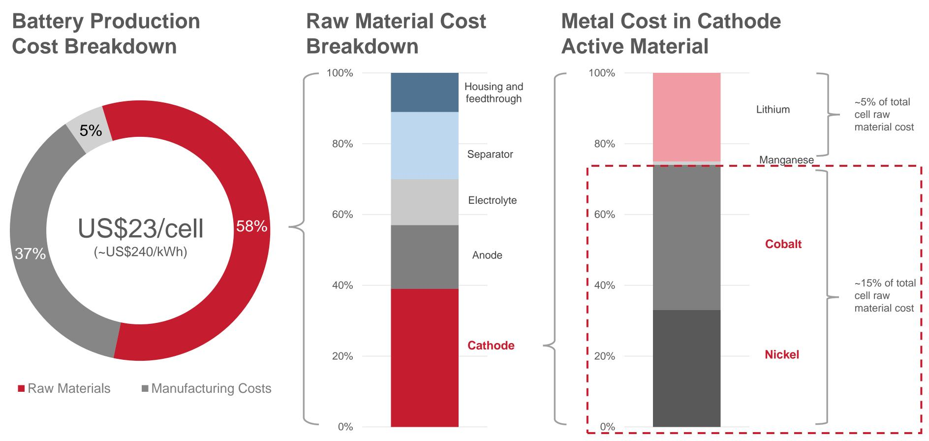
Source: Roland Berger (2012) and internal analysis. Assumes a 96Wh PHEV cell (26Ah, 3.7W) using NCM622 cathode chemistry. Cathode raw material cost includes non-metallic materials (carbon black, binder, foil). Internal assumptions concerning split of costs assumes spot prices of Ni US\$4.20/lb; Co US\$28.00/lb; Mn US\$1.00/lb; Li US\$9,000/t (as LCE)
