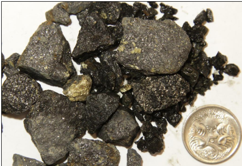
Figure 3. Examples of variably disseminated sulphides within magnetite, CRC001-008.
