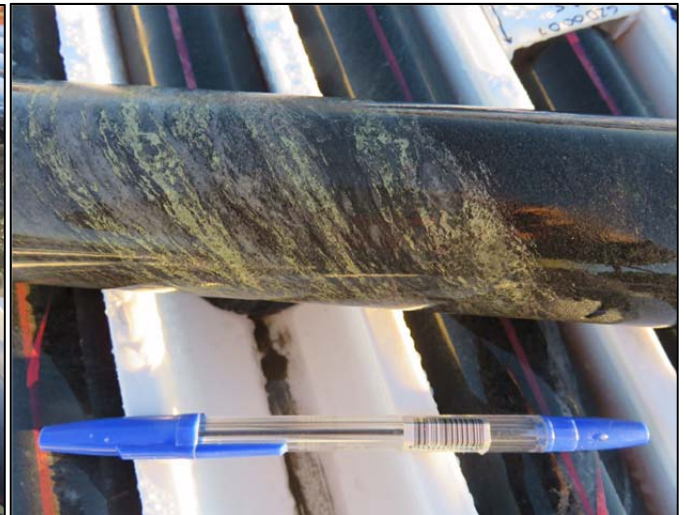
Figure 2. High grade matrix sulphide at 614m.
