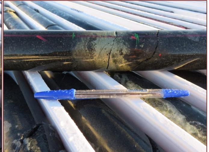
Figure 4. Chalcopyrite-rich stringer at 599m.
