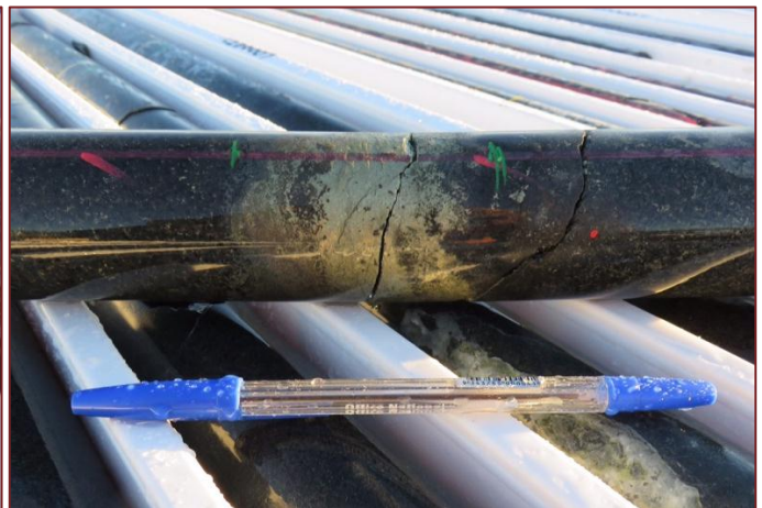
Figure 2. High grade veinlet of chalcopyrite (14.1% Cu) at 599m.
