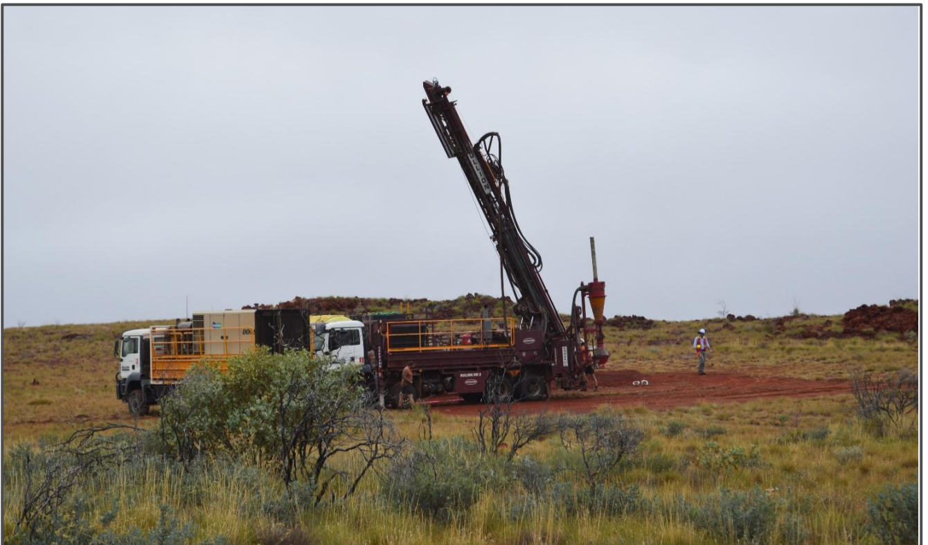
Figure 1. RC drilling commencing at the Iapetus Prospect. Gossan outcrop in background.
