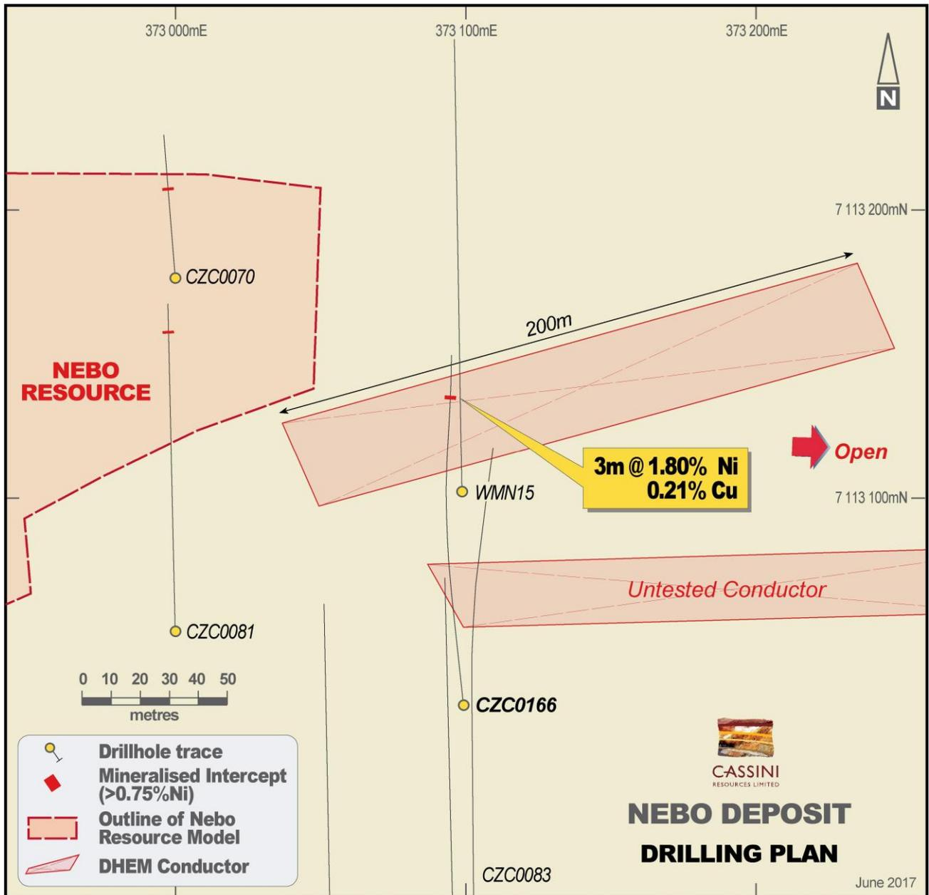
FIGURE 1. Nebo Deposit plan showing target conductors and hole CZC0166.
