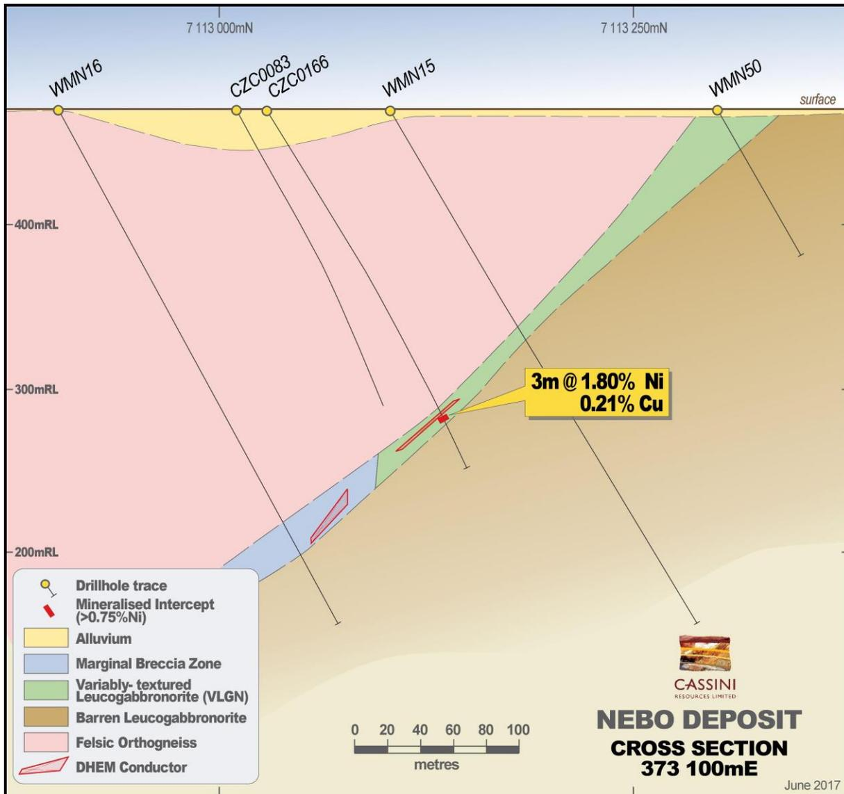
FIGURE 2. CZC0166 cross-section.
