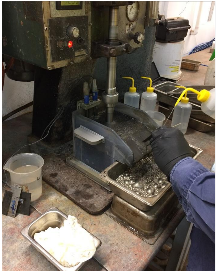
FIGURE 1. Float testing of West Musgrave samples
