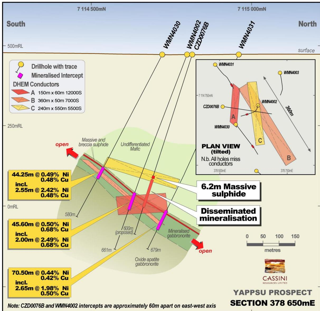
Figure 4. Yapsu section and plan showing approximate intersections in CZD0076B.
