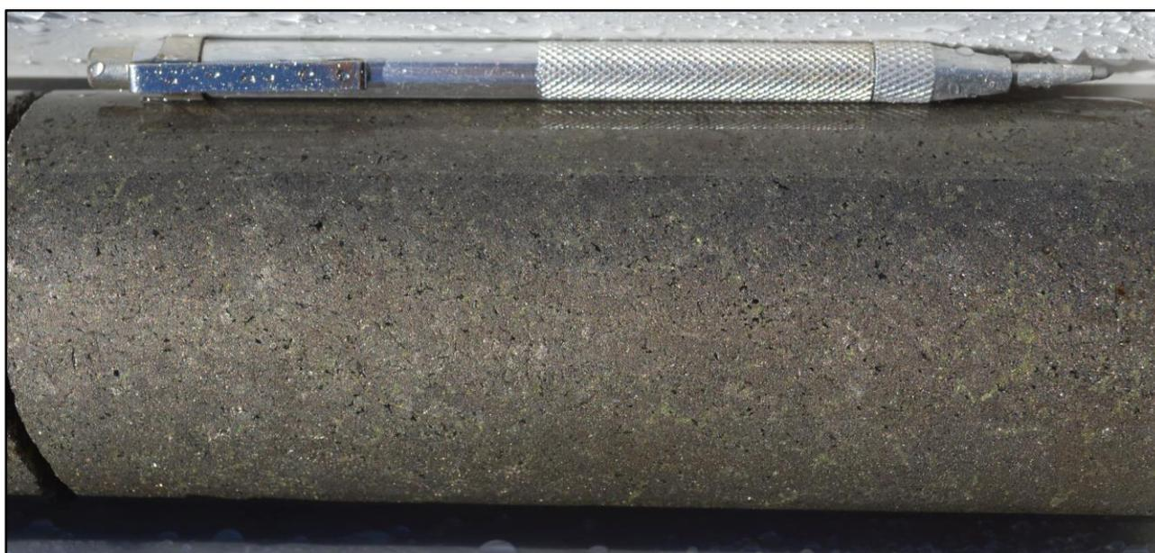
**Figure 2.** Massive sulphide mineralisation at 429.1m, CZD0076B.
