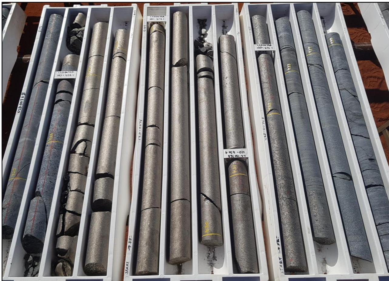
**Figure 1.** Massive sulphide mineralisation (golden coloured core) from upper zone, CZD0076B.
